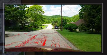
RoadBotics by Michelin artificial intelligence, through its machine learning process, scans high-resolution image data on a pixel-by-pixel basis to recognize road distresses a trained engineer would look for when conducting a visual survey. After identifying those distresses, a 1-5 condition rating is automatically generated to score the quality of each 10-foot section of road.
